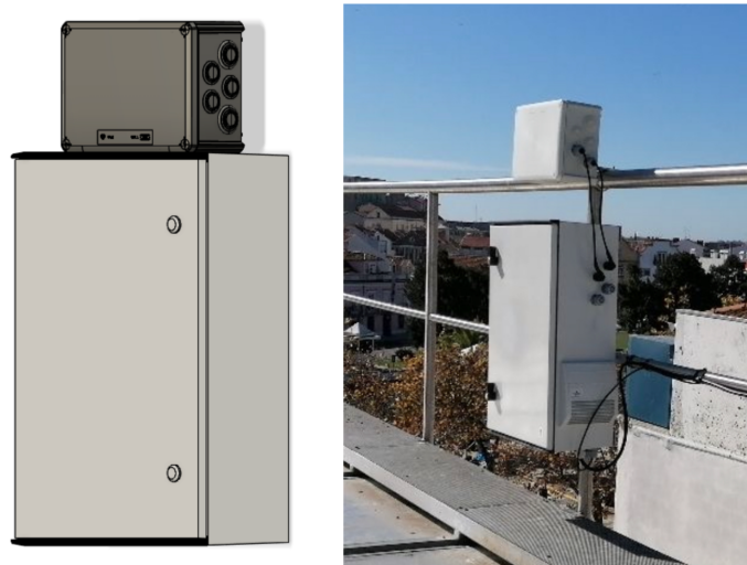
Figure 2.9: Wall Boxes. Design and deployment in the city
