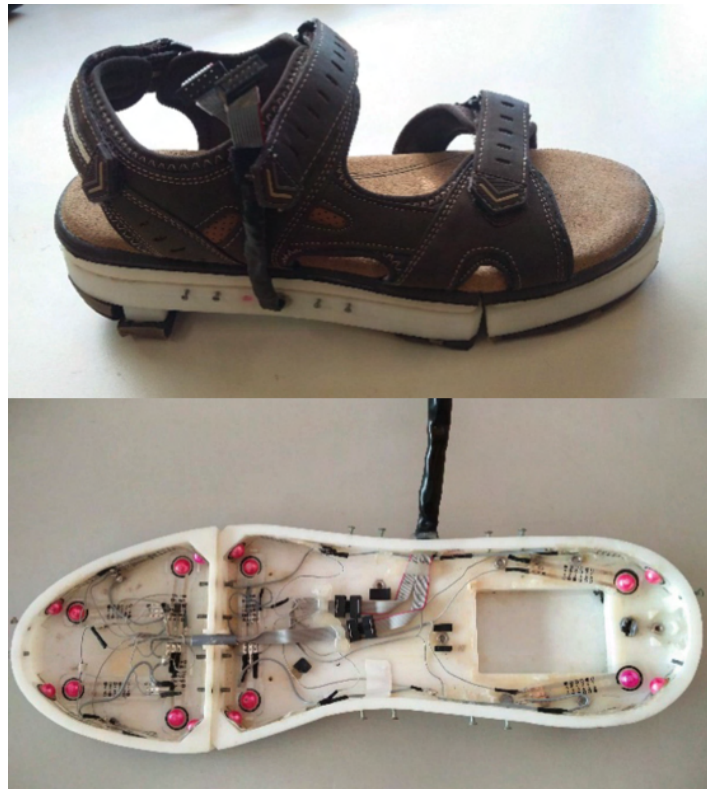
Figure 2.9: Example of an instrumented shoe prototype (adapted from [10]).
