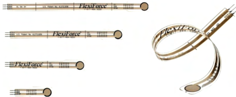
Figure 2.8: Example of a Tekscan FlexiForce pressure sensor (piezoresistive) (taken from [44]).
