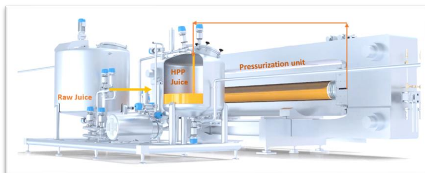
Figure 2.5 - Schematic representation of a HPP bulk unit (adapted with permission from Hiperbaric, Spain).
