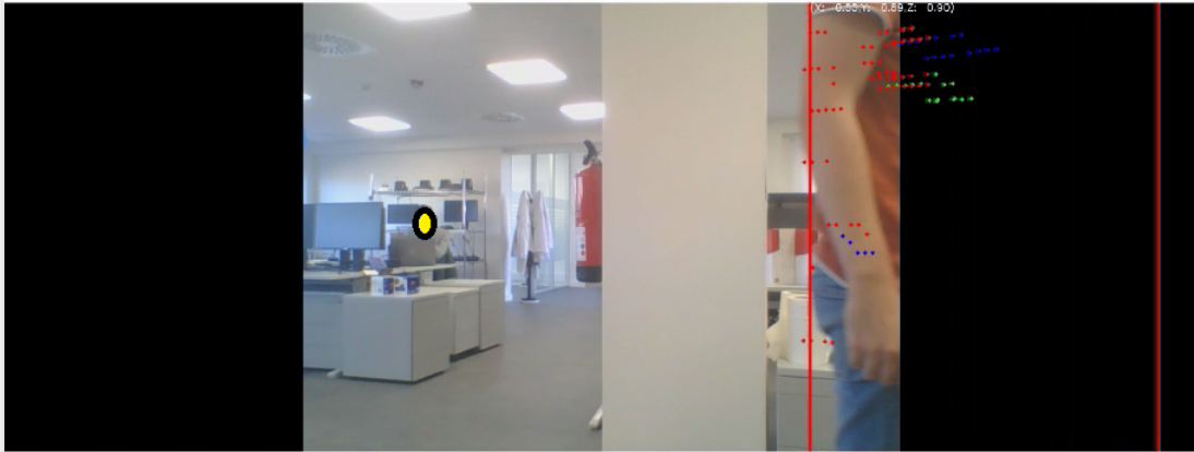
Figure 5.8: Target moving out of camera vision but still in radar FoV.
