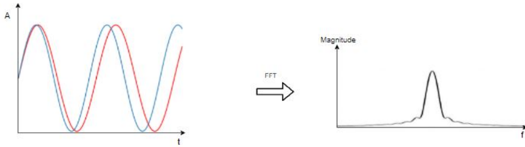
Figure 2.8: The amplitude-time plot (left) of the IF signals of two targets at very close distance. At the right plot is the FFT of the IF signals with a small observation time window with just N samples. Adapted from [10].
