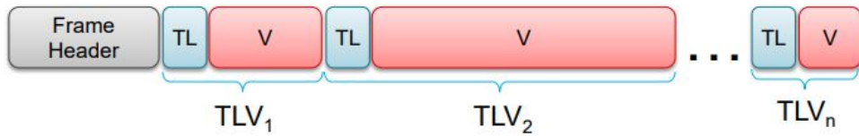
Figure 3.18: Data Packet structure sent to PC with multiple TLV blocks from a single packet. From [9].
