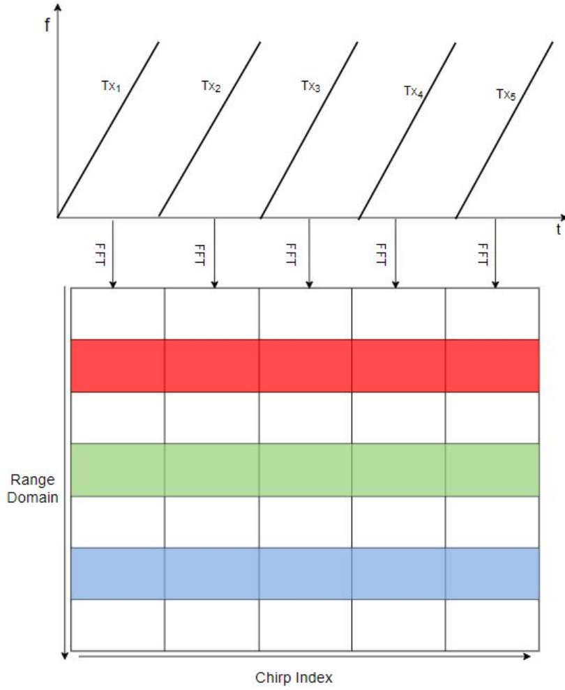
Figure 2.7: The 1D-FFT or range-FFT.
