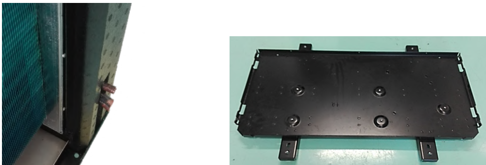
(a) Evaporator refrigerant lines and EPP opening.
