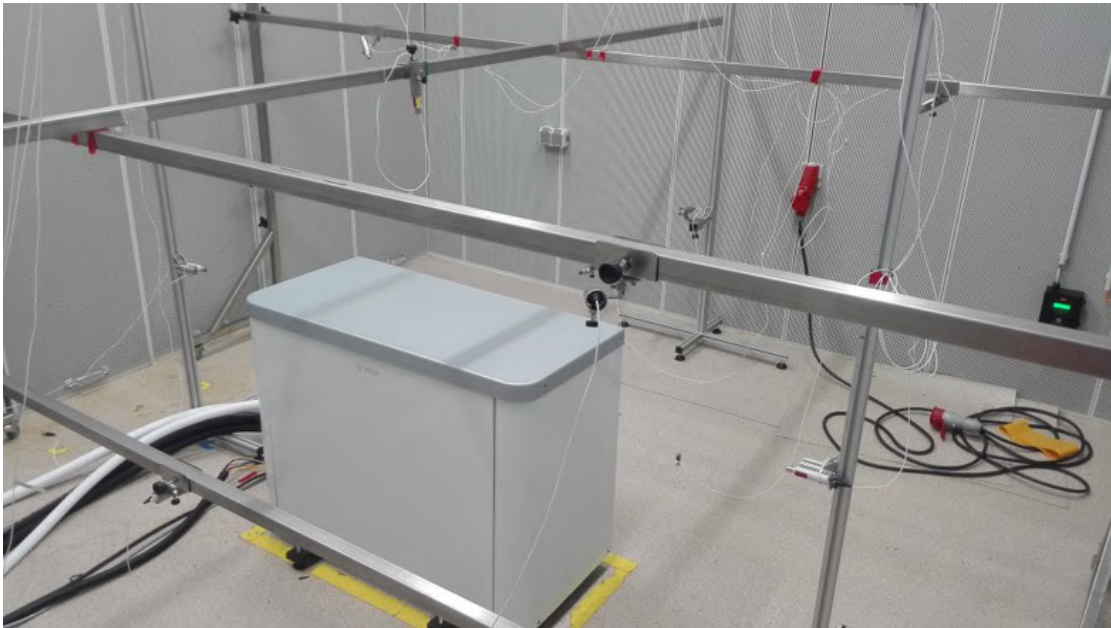
Figure 6.3: Sound measurement set-up accordingly to ISO 3744.
