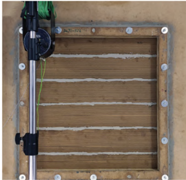
Figure 2.2: Experimental setup of the WPC panel composed by 6 boards [23].
