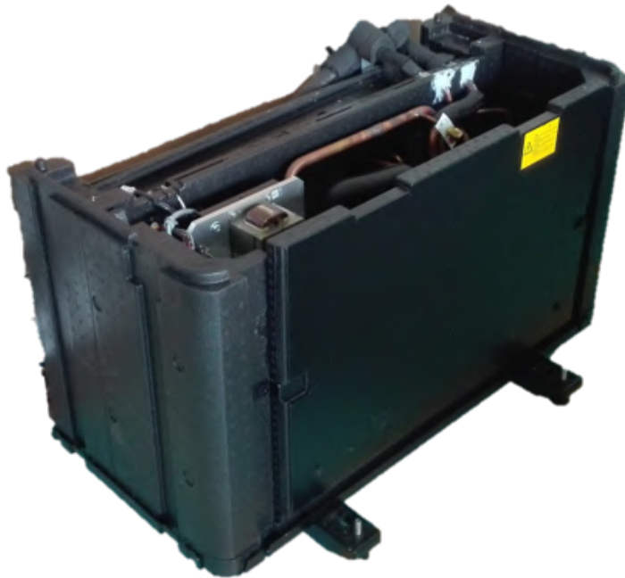
Figure 4.5: Compressor module - EPP structure without lid.
