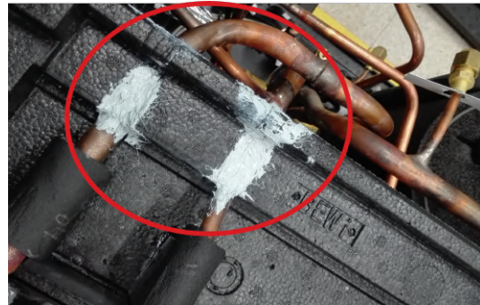
(b) Sealing of the EPP holes through which the refrigerant lines run.
