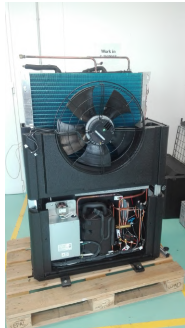
(b) AirX 90 - partially disassembled EPP structure.
