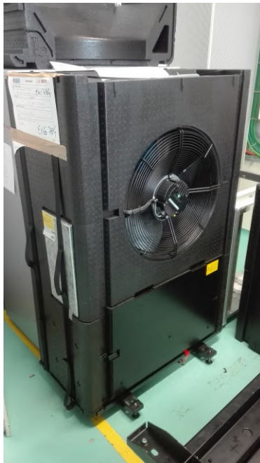
(a) AirX 90 - EPP structure.
