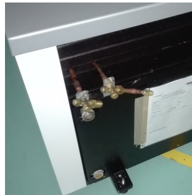
(b) CM - shut-off valves installed.
