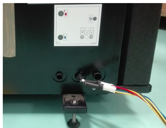
(b) Compressor module - wiring exists.
