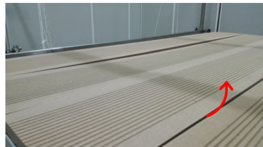
(b) Sound leakage between WPC boards on the top face.
