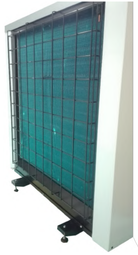
Figure 4.18: Fan module - evaporator with the protection grid installed.
