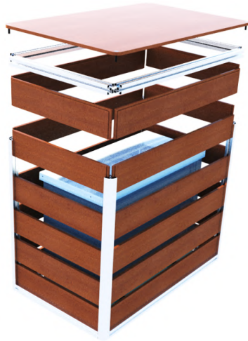
(a) 3D CAD design - exploded view.
