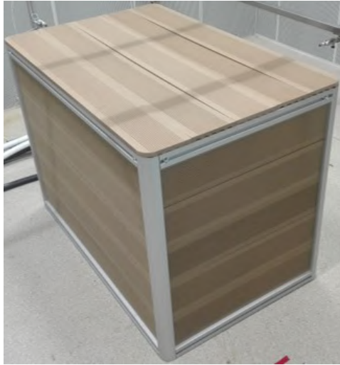
(a) WPC acoustic enclosure installation around the compressor module.
