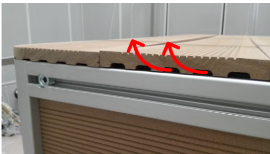
(a) Sound leakage through the lateral openings of the WPC boards.
