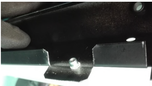
(a) Re-work of the grid support.
