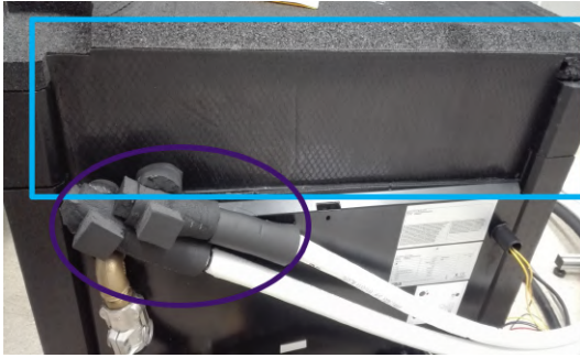
(a) In blue - addition of a bitumen layer on the top rear EPP part of the compressor module; In purple - addition of foam around the shut-off valves.
