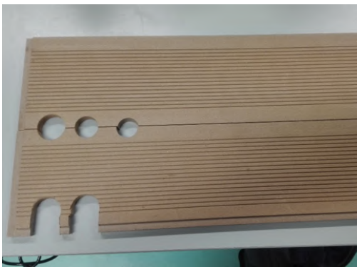
(a) Detail of the holes drilled in the WPC boards to allow the water and refrigerant hoses and the electrical extensions to pass through.
