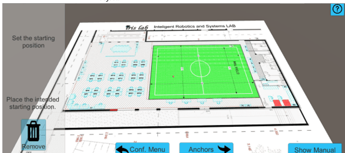
(b) Desktop PC configuration UI for positioning the virtual object representing the smartphone starting position.
