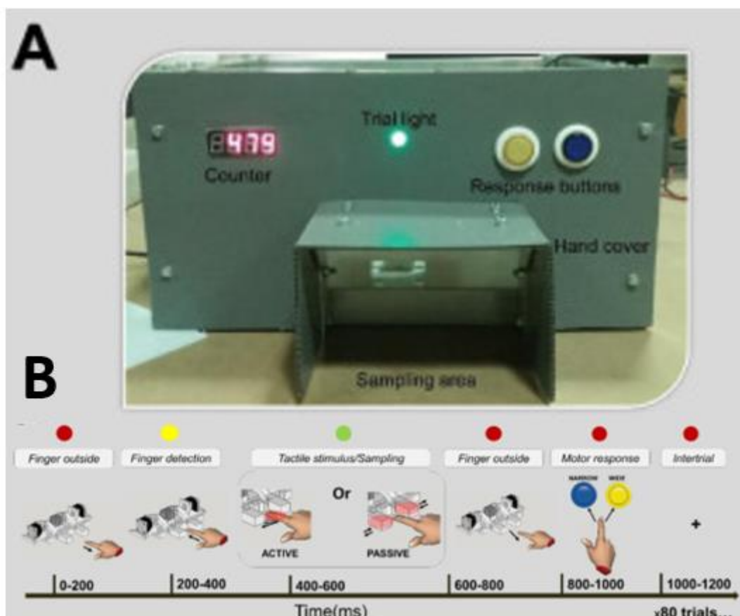
Figure 6. Device and experimental design of the active touch experiment. A) Device used during the trial B) Process followed by the subject during each trial adapted from "Differential width discrimination task for active and passive tactile discrimination in humans"
