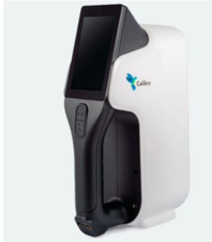
Figura 5.2: Scanner com feixe de luz estruturada, Calibry ( https://thor3dscanner.com/en/products/ )
