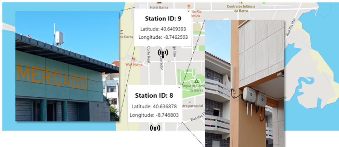
Figure 4.14: RSUs installed with a fiber connection
