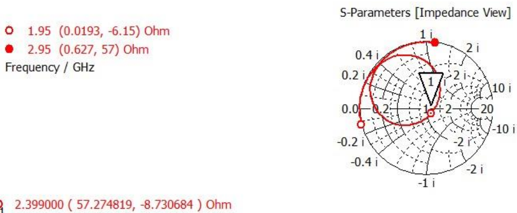
Figure 19: Smith Chart representation of the S_{11} of the microstrip line fed rectangular patch with quarter-wavelength transformer.
