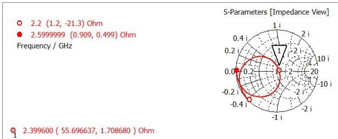
Figure 38: Smith Chart representation of the S_{11} of the aperture coupled line fed circular patch with rectangular slot.
