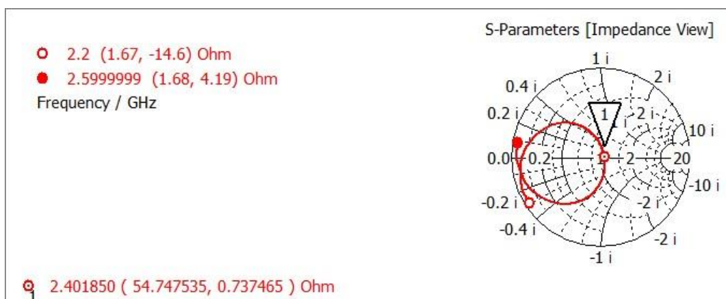
Figure 27: Smith Chart representation of the S_{11} of the proximity coupled line fed rectangular patch.
