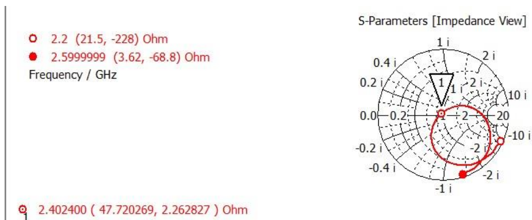
Figure 29: Smith Chart representation of the S_{11} of the proximity coupled line fed circular patch.
