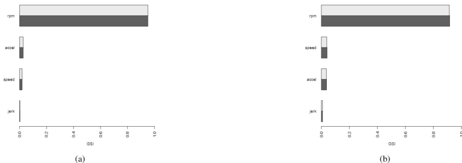
Fig. 3: GSI for: (a) route A1 and (b) vehicle V1. The pale bars corresponds to the average main effects and the dark bars to the total effects.
