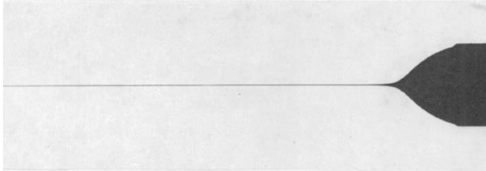
Figure 6: Image of a jet of glycine with the formation of Taylor cone 59 .
