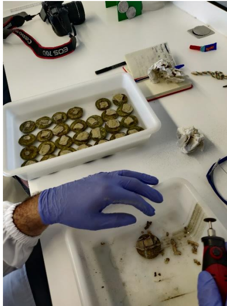
Figure 2 – Fragmentation process of M. capricornis using the Einhell Grinding and Engraving tool
