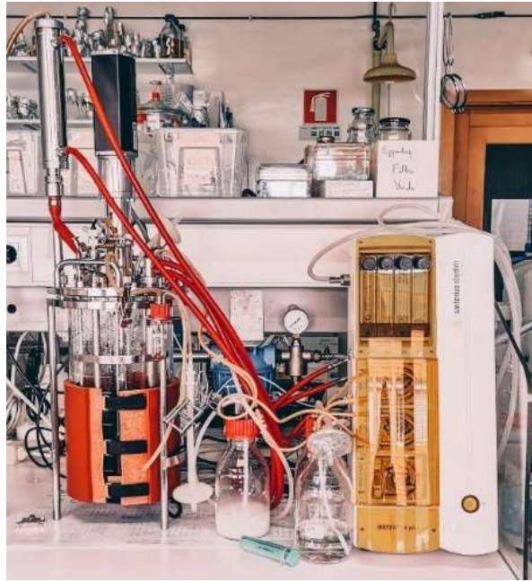
Figure 10 - Sartorius Biostat A plus reactor used for the assays with C. necator DSM 545.
