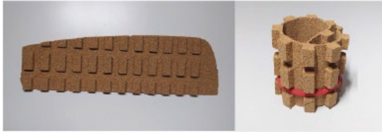
Fig. 61 - Flexibility of a 10 mm piece of cork machined 7.5 mm deep
