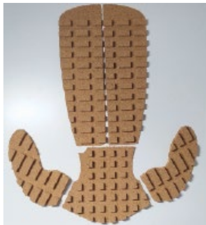
Fig. 60 - Separate pieces of cork before being glued to a piece of fabric with the shape of the whole
