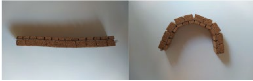
Fig. 59 - Several pieces of cork glued to a piece of fabric and how it affects the bending of the entire system
