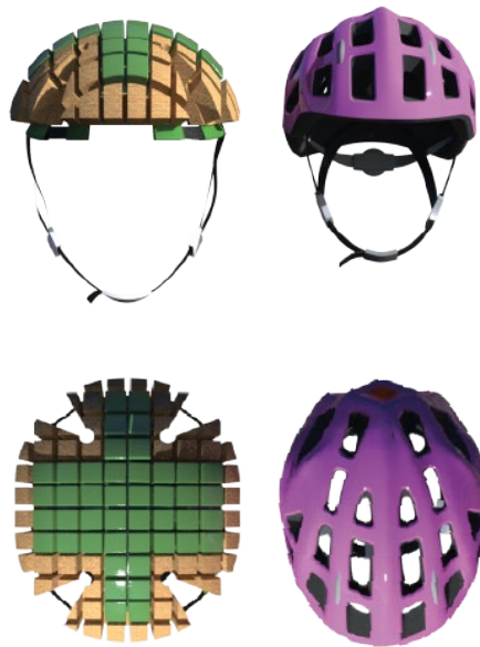
Fig. 77 - Helmet models used to obtain volumetric data for LCA comparison. On the left, the concept's model and, on the right, the model from GrabCad (2021).
