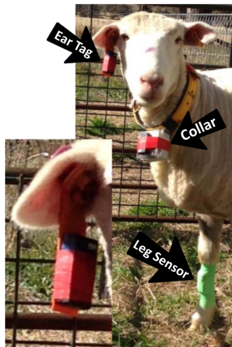
Figure 3.2: Distinction between a collar, an ear tag and a leg sensor [194].
