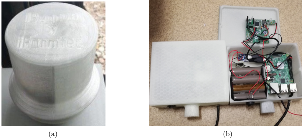
Figure 8.2: (a) Beacon prototype; (b) Gateway prototype.
