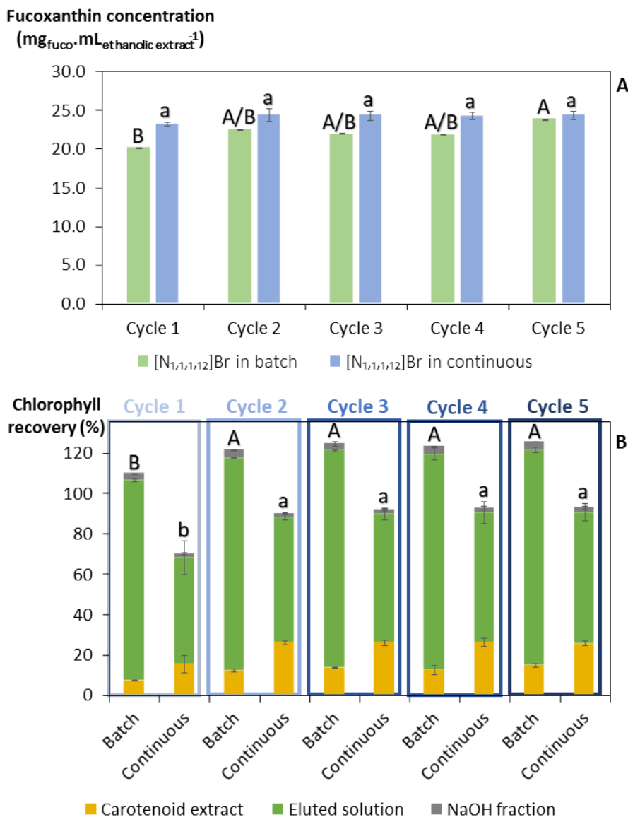
Figure 2.1.7. Comparison of the process using an aqueous solution of [\text{N}_{1,1,1,12}]\text{Br} as eluent both in batch and in continuous regime along five cycles of reuse of the resin, considering (A) fucoxanthin concentration in the carotenoid ethanolic extract (first fraction collected from the resin); and (B) chlorophyll recovery in the different fractions collected from the resin. Results regarding the batch process are once more displayed to facilitate the comparison. Note that different initial values in (A) are due to the need of preparing new initial extracts in the beginning of each experiment. Capital letters represent statistically results in the process mediated by [\text{N}_{1,1,1,12}]\text{Br} in batch ( p < 0.05 ). Lowercase letters represent statistically results in the process mediated by [\text{N}_{1,1,1,12}]\text{Br} in continuous ( p < 0.05 ).
