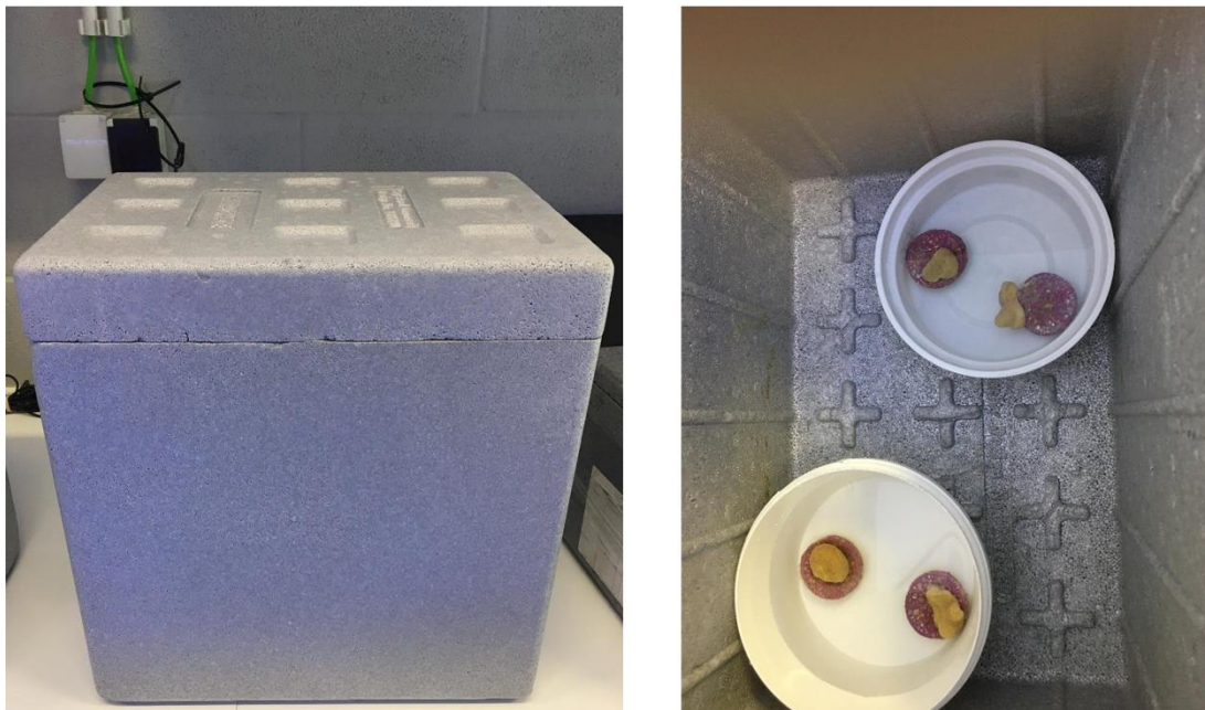
Figure 21 - Styrofoam box employed to perform dark-adaptation of fragments of Sarcophyton cf. glaucum before performing PAM fluorometry readings.
