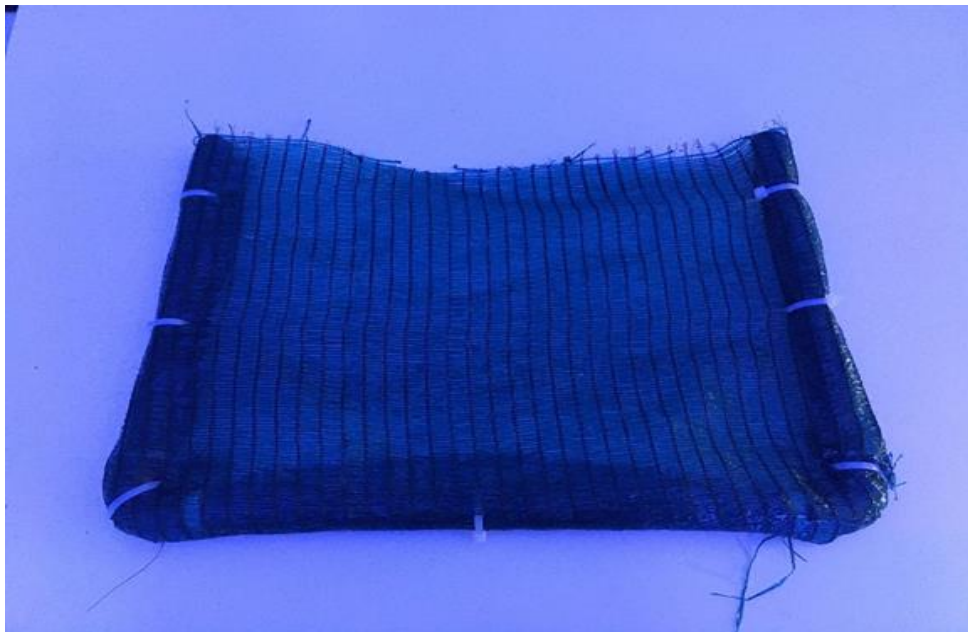
Figure 16 - Shading frame used to achieve a LL intensity in one part of the tanks.
