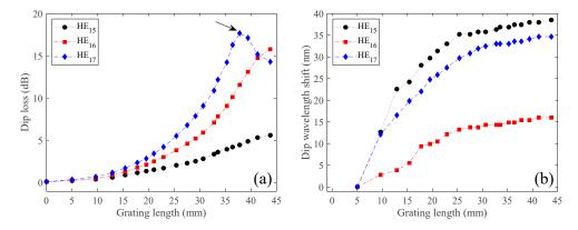
**Figure 7.** (**a**) Dip attenuation and (**b**) dip wavelength shift as function of the grating length, obtained for the LPG grating spectra shown in Figure 6.
