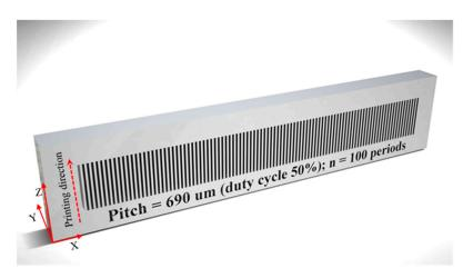
Figure 1. CAD (computer aided design) image of the 690 μm amplitude mask.
