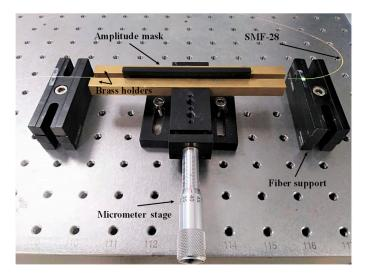
Figure 3. Setup used to mechanically induce LPGs in a standard optical fiber.
