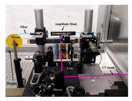
**Figure 2.** Picture of the setup used for the UV inscription of long-period gratings (LPGs) through the amplitude mask technique. The laser beam is guided through mirrors, focused by a cylindrical lens, passing through the 3D printed amplitude mask and hitting the optical fiber behind. The weight on the fiber is used to keep the same fiber strain between experiments.
