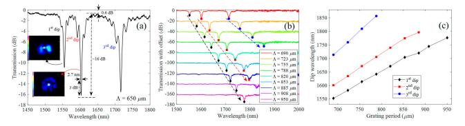
**Figure 10.** LPG transmission spectra acquired with the pressure induced method for a 3D printed amplitude mask with: (**a**) 690 μm period and (**b**) 690–950 μm periods. The insets shown in (**a**), are the experimental near-field profiles of the 1st and 2nd dip resonances. The screw displacement was set to induce the deepest mode losses. (**c**) Dip wavelength shift as function of the grating period for the different LPG resonances seen in (**b**).
