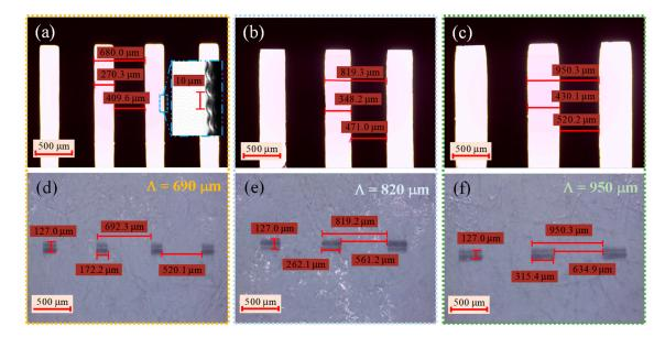
**Figure 5.** Microscope images of the amplitude masks (**a**–**c**), and the UV pattern imprinted in a thermal paper using those masks (**d**–**f**). Top images correspond to the periods of: 690  $\mu$ m (**a**,**d**), middle images to the 820  $\mu$ m (**b**,**e**), and bottom images to the 950  $\mu$ m (**c**,**f**).
