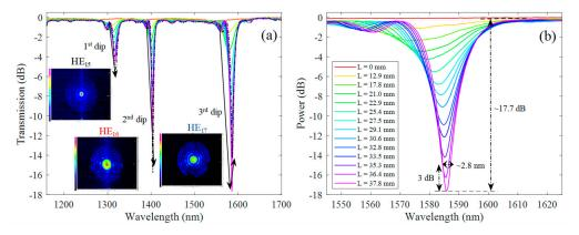
**Figure 6.** (a) LPG transmission spectra over time (i.e., as the grating length increases), obtained using the amplitude mask technique, by scanning a UV laser beam with velocity of 125  $\mu$ m/s along a 690  $\mu$ m period amplitude mask. The inset shows the experimental near-field profile of the modes corresponding to the attenuation dips. (b) Inset of the 3rd transmission dip (HE<sub>17</sub> mode) as function of the grating length.
