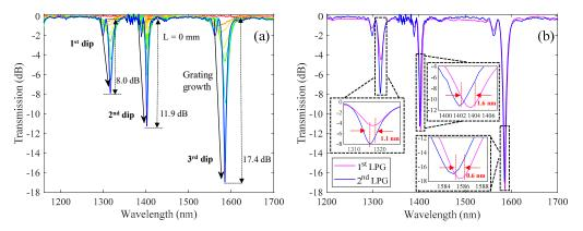
**Figure 8.** (a) Transmission spectra acquired during the grating inscription, for an LPG written with the same conditions as the one presented in Figure 6, (i.e., scanning the UV laser beam (E = 3.9 mJ, R = 500 Hz), with velocity of 125 µm/s along a 690 µm period amplitude mask). (b) Transmission spectra of two ~38 mm LPGs, either from the results collected in Figure 6 (1st LPG) and for a new grating with similar writing parameters (2nd LPG).
