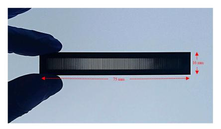
Figure 4. Picture of the 3D printed amplitude mask.
