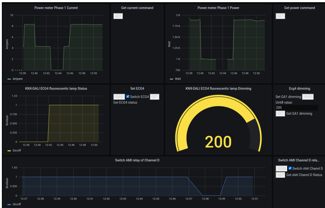
Figure 5.14: Part of the KNX Device Dashboard.
