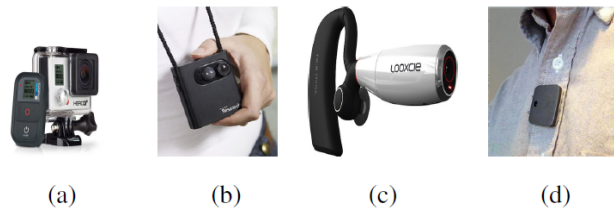
(a) a)GoPro b)SenseCam c)Looxcie d)Narrative Clip[20].
