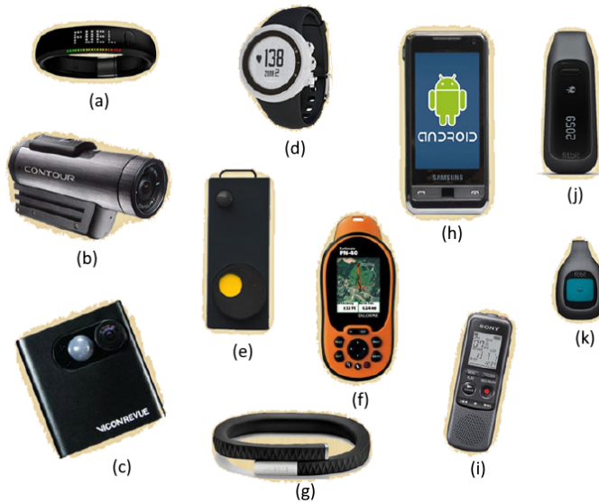
(b) a) Nike ‘Fuelband’, b) Contour wearable video camera with GPS, c) Vicon Revue wearable camera with sensors, d) Heart Rate Monitor display watch, e) Autographer from Vicon, f) GPS tracker, g) Jawbone’s ‘Up’ Fitness Tracking Bracelet, h) Smartphone with built-in sensors, i) Audio recorder, j) fitbit ‘One’ Wireless Activity Tracker, k) fitbit ‘Zip’ Wireless Activity Tracker[21].
