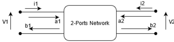
Figure 4.2: S-Parameters network of two-ports with incident and reflected waves.
