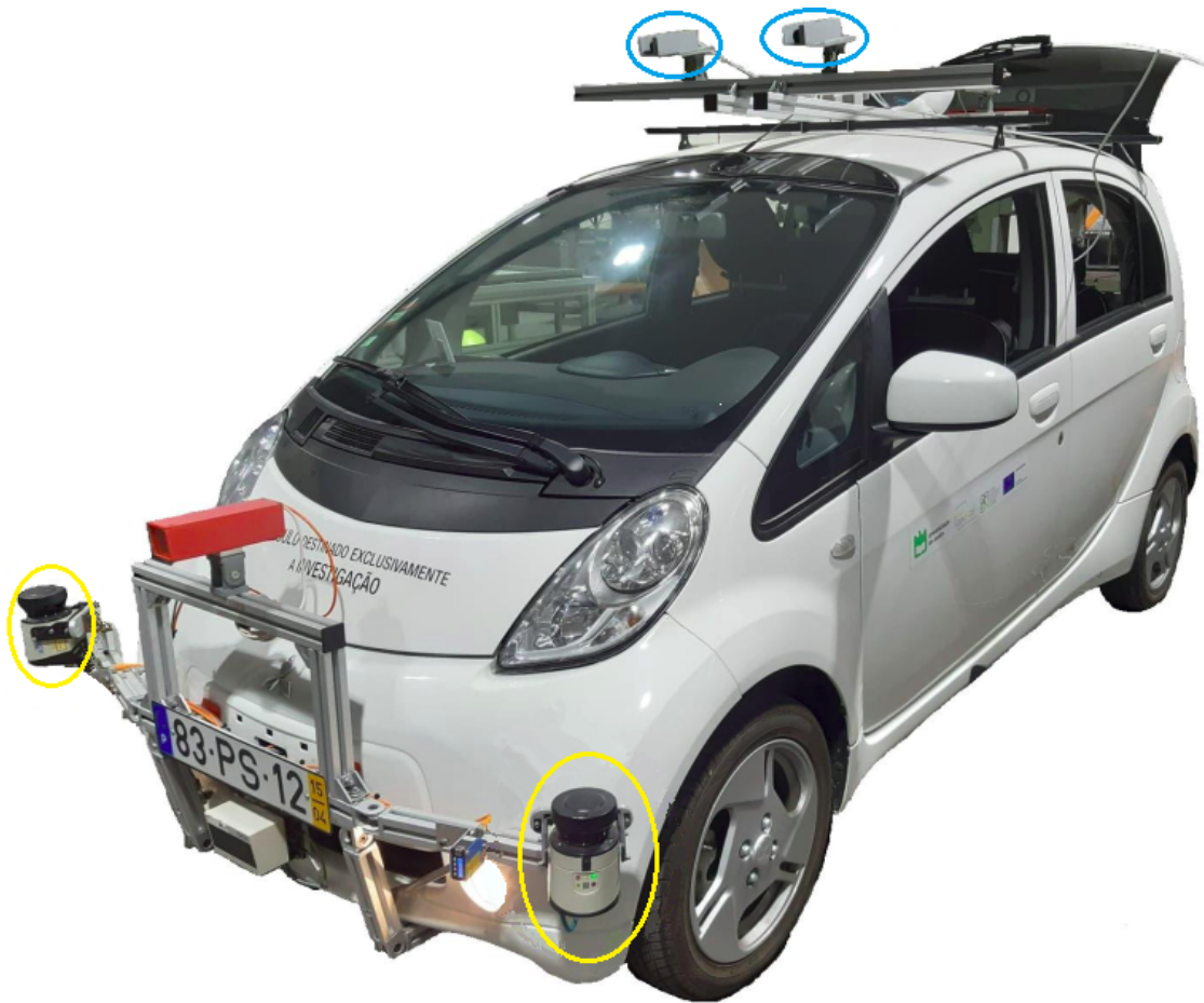
Figure 5.2: ATLASCAR2 with the LiDAR sensors circled in yellow and the cameras in blue.
