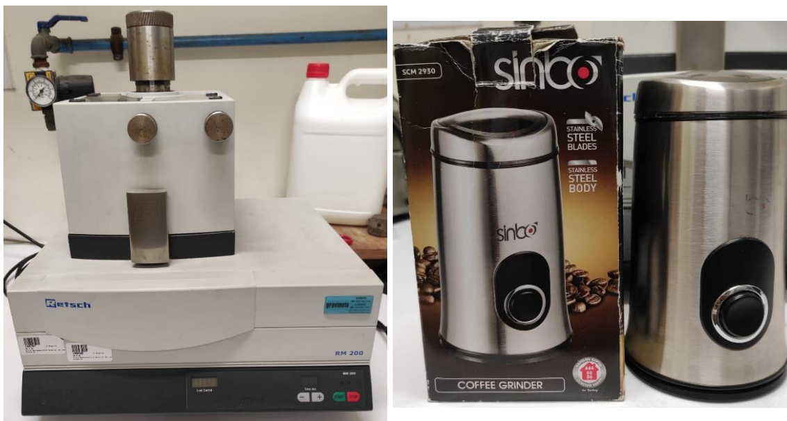
Figure 6: Retsch RM 200 mortar grinder (left picture) and SCM 2930 coffee grinder (right picture) used to homogenize food samples
