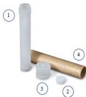
Figure 12: MarsXpress™ vessel that is composed by a liner (1), a vessel plug (2), a cap (3), and a sleeve (4)
