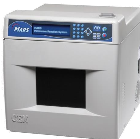
Figure 14: Microwave oven, model CEM Mars 5 240/50, used for the digestion of samples
