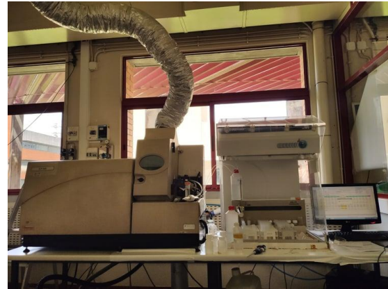
Figure 5 – Inductively coupled plasma mass spectrometry (ICP-MS) – Thermo ICP-MS XSeries equipped with a Burgener nebuliser.
