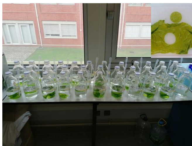
Figure 7 – Set up of the preliminary study of Hg, Co and Ni removal. On the top right corner it is represented the disks of macroalgae used in the essay.
