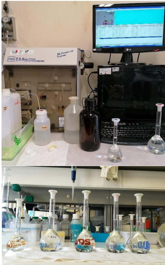
Figure 4 - Cold vapour atomic fluorescence spectroscopy (CV-AFS) (top) and daily standard solutions (bottom).
