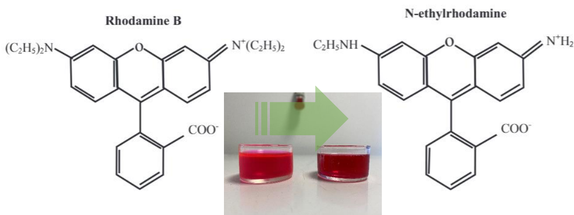
Fig. 4. 2. Possible transformation product of RhB when a thermal activation was used to generate the oxidation agents from PS under the operating condition of [PS]_0=5 mM, CuO=0.0 g/L, pH=7 and temperature= 45 °C.
