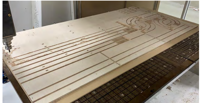
fig.79: CNC machining the prototype components.
