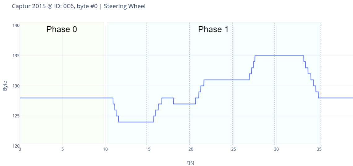
Figure 5.15: Graphic with the variations of the steering wheel in byte #0 of the CAN message with ID 0C6 over the time
