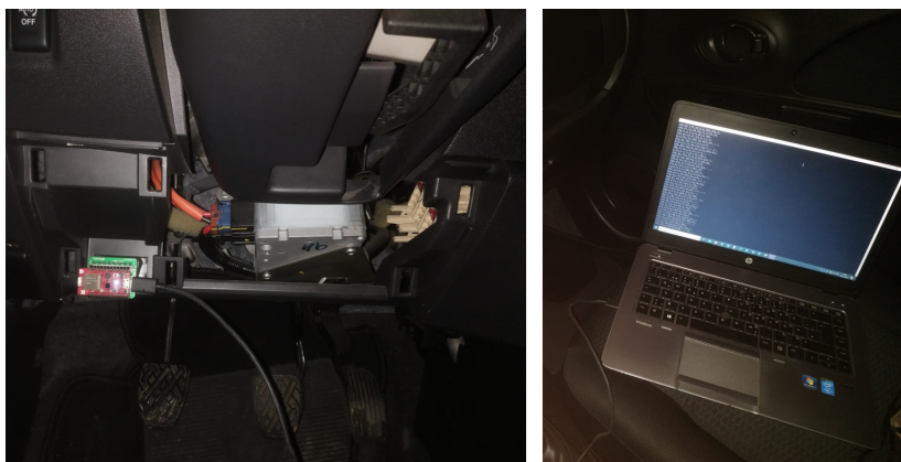
Figure 5.5: Setup with Carloop and PC in Nissan Micra 2012
