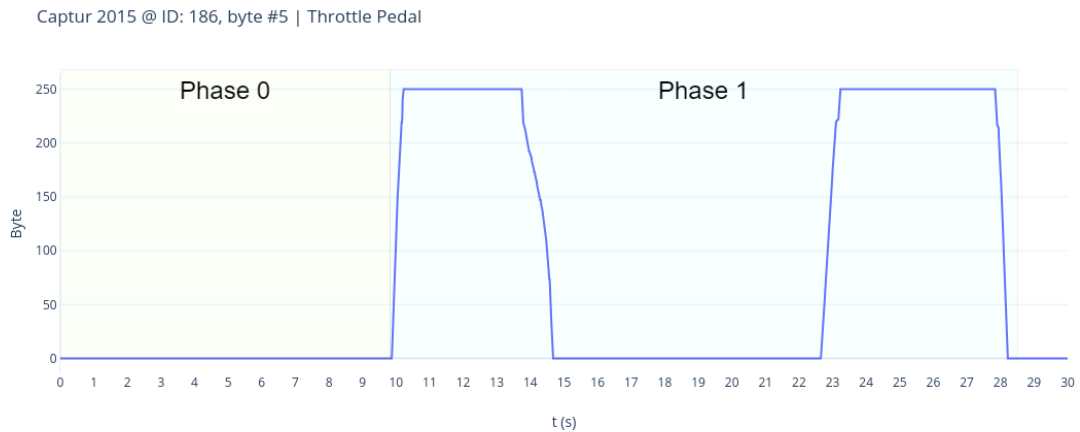
Figure 5.17: Graphic with the variations of the throttle pedal in byte #5 of the CAN message with ID 186 over the time
