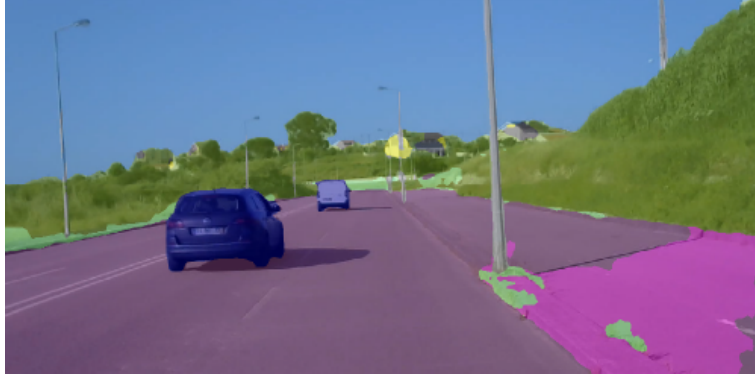
Figure 5.9: Example of poor detection of the sidewalk. In this case, the model detects a part of the sidewalk correctly, however it does not detect the continuation of that sidewalk after the pole. This could lead to a collision, since the car could assume that it should switch to the lane further to the right.
