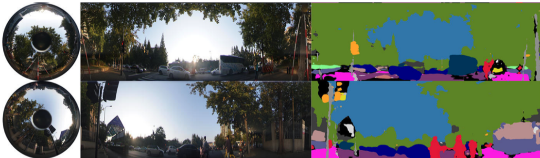
Figure 2.22: Results of the segmentation of panoramic images presented in [45]. The first picture is a raw panoramic annular image, the middle one is the unfolded panoramic image and the last one is a segmentation map.
