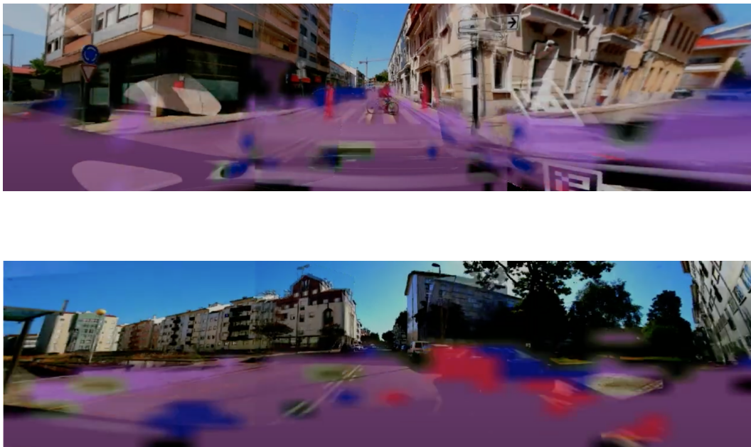
Figure 5.13: Tests performed on board ATLASCAR2. The first image is relative to the panoramic created by merging the segmented images and the second image is the result of the segmentation of the panoramic image.
