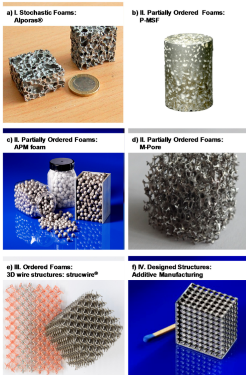
Figure A.3: Exemplary images of the different foams' classes, which illustrate the level of order and structural control [30]. a) Alporas foam; b) P-MSF foam; c) APM foam; d) M-Pore foam; e) Structwire; Additevely manufactured 3D lattice structure.
