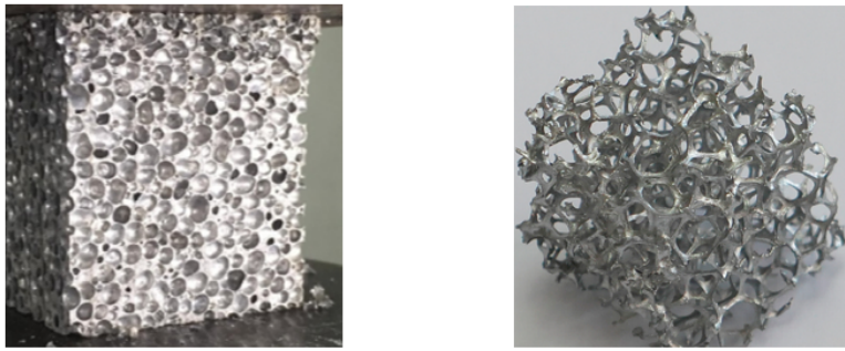
Figure 2.1: Closed-cell (left) and open-cell foam specimens [33, 34].
