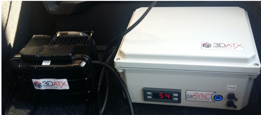
Figure 3.6: 3DATX iPEMS (white) and the Water Trapper (black) devices
