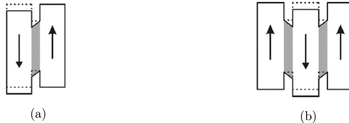
Figure 1.6: (a) One-sided shear test specimen and (b) shear test specimen according to Miyauchi [Brosius et al. 2011].
