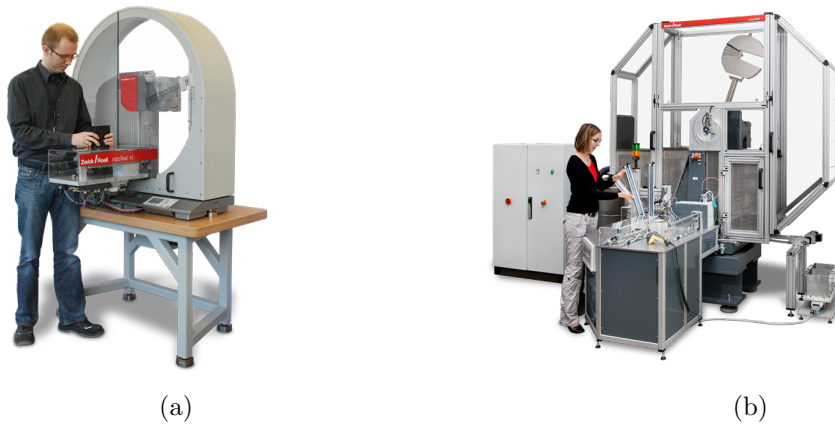
Figure 3.6: (a) Robotic testing system RoboTest H and (b) RoboTest I [12].
