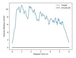
(b) Target velocity as detected by the GNN (in blue) and ATLASCAR2 velocity (in black) during the experiment.
