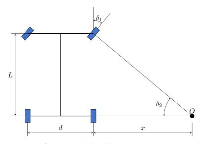
Figure 5.1: Schematics of the Ackermann steering geometry.
