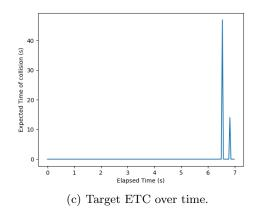
Figure 6.20: Graphic representation of distance, velocity and ETC data collected while the passenger vehicle drove towards a tail collision with the ATLASCAR2.
