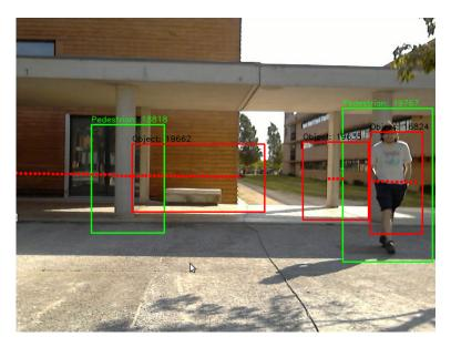
Figure 2.1: Sensor Fusion LIDAR-Camera with LIDAR detected objects in red dots [5].
