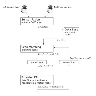
Figure 2.5: A LIDAR based ego-motion estimation setup [15].
