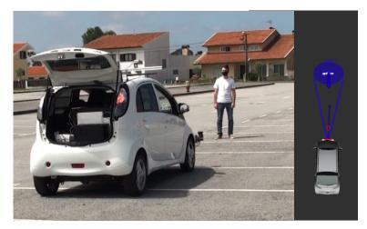
Figure 6.2: Front collision setup on the left and on the right the Rviz visualization of the VO cone (the blue lines) as well as the enlarged target circle .
