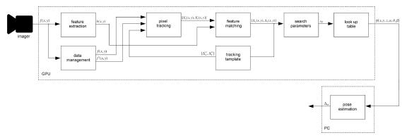
Figure 2.4: A Visual Odometry set up [16].
