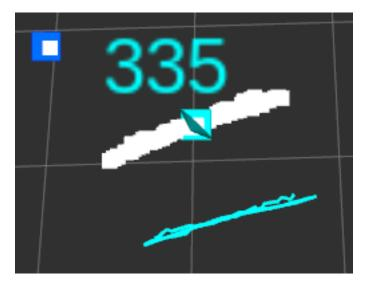
Figure 4.3: Representation errors due to old point data. The target first detection is represented by the cyan line. The target then moved, however the line position was not updated.
