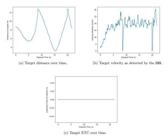
Figure 6.9: Graphic representation of distance, velocity and ETC data collected while rotating around a static target placed on the outer side of the turn.
