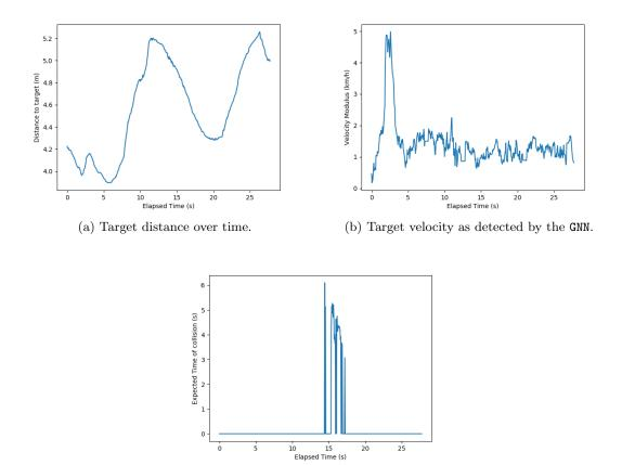
Figure 6.8: Graphic representation of distance, velocity and ETC data collected while rotating around a static target placed on the car's turning center point.
