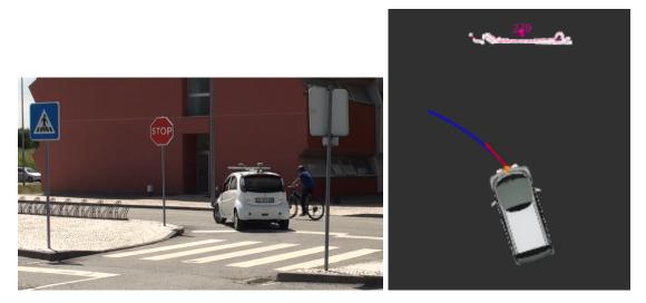
Figure 6.12: On the left an image of the experiment, in this case with a bicycle portraying the dynamic target; On the right the Rviz representation of the data collected using a passenger vehicle. The target is represented in pink with id 279, the ATLASCAR2 short term path in blue and the instantaneous velocity vector in red.
