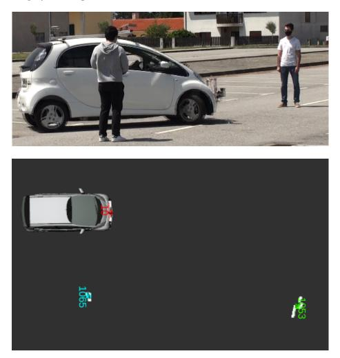
Figure 6.6: On the top an image of the Rotating Around Two Pedestrians experiment; On the bottom the Rviz representation . The target placed in the turning center point is represented in cyan with id 1065 and the pedestrian placed outside the turn in green with id number 1053.
