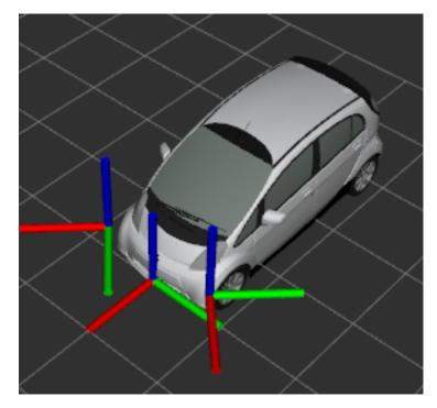
Figure 4.5: The ATLASCAR2 relevant frames; From left to right: *Right\_laser*, *base\_link*, *left\_laser*.
