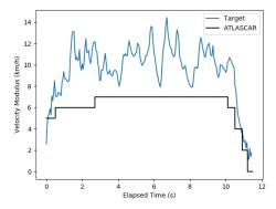
(b) Target velocity as detected by the GNN (in blue) and ATLASCAR2 velocity (in black) during the experiment.
