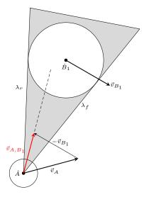
Figure 4.1: "Collision Cone"  $CC_{A,B}$  represent by the gray area. Adapted from [9].
