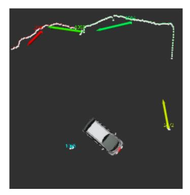
Figure 6.7: Rviz representation of the Rotating Around Two Pedestrians experiment error. The target placed in the turning center point is still being tracked with the same id 1065, however the target outside th8 turn (id number 1053) is being embraced by the background measurements, causing the target to merge with the remaining points and therefore lose the pedestrian tracking.
