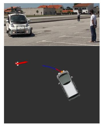
Figure 6.4: Image of the experiment of the After Turn Collision experiment on the top; On the bottom the Rviz representation of the target to be collided with in red with id number 0, the ATLASCAR2 short term path in blue and the instantaneous velocity vector in red.
