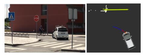
Figure 6.14: On the left an image of the experiment, in this case with a bicycle portraying the dynamic target; On the right the **Rviz** representation of the data collected using a passenger vehicle. The target is represented in yellow with id 312, the ATLASCAR2 short term path in blue and the instantaneous velocity vector in red.
