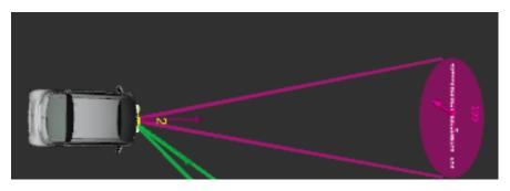
Figure 6.16: Rviz representation of the ATLASCAR2 sideways collision experiment with the target id 199. The collision cone can also be seen with the pink lines as well as the enlarged target circle.
