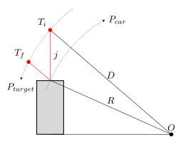
Figure 5.4: Example of a static target  $\,T$  while the ATLASCAR2 is performing a right turn.
