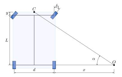
Figure 5.2: Schematics of the Ackermann steering geometry.
