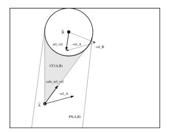
Figure 2.2: "Relative Collision Cone" CC(A,B) [7].
