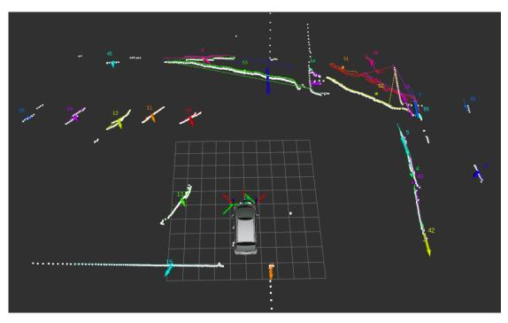
Figure 3.3: Rviz environment displaying the ATLASCAR2 robot model, the LIDAR laserscan, and several markers of the targets.
