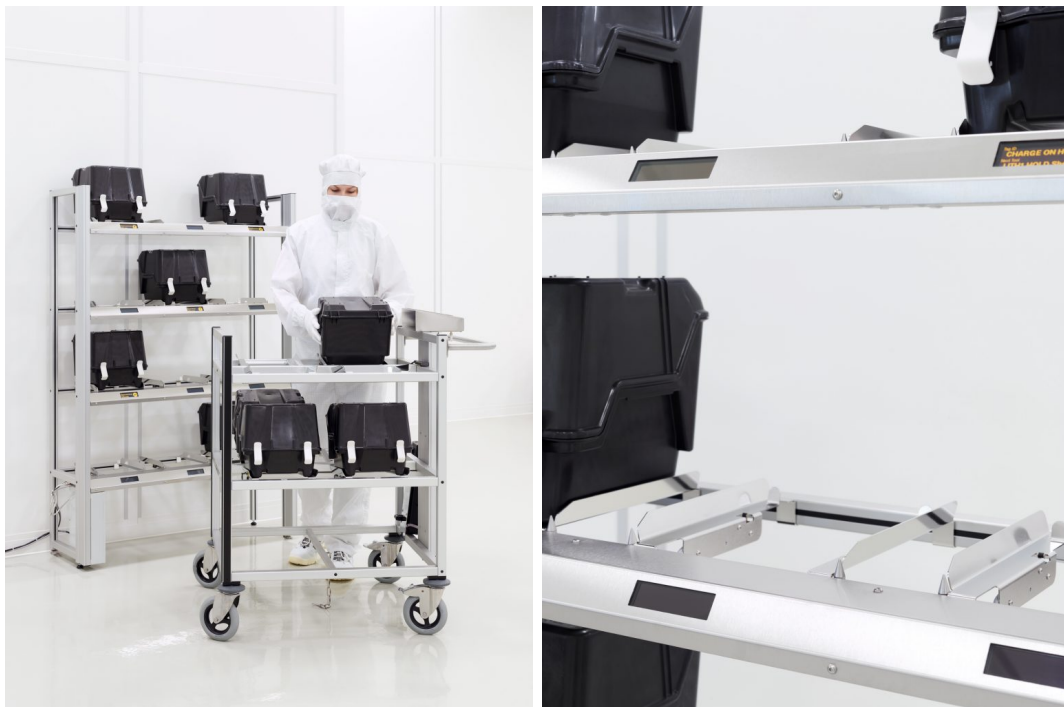
Figure 4.3: Fabmatics RFID Rack design for wafer storage [100]
