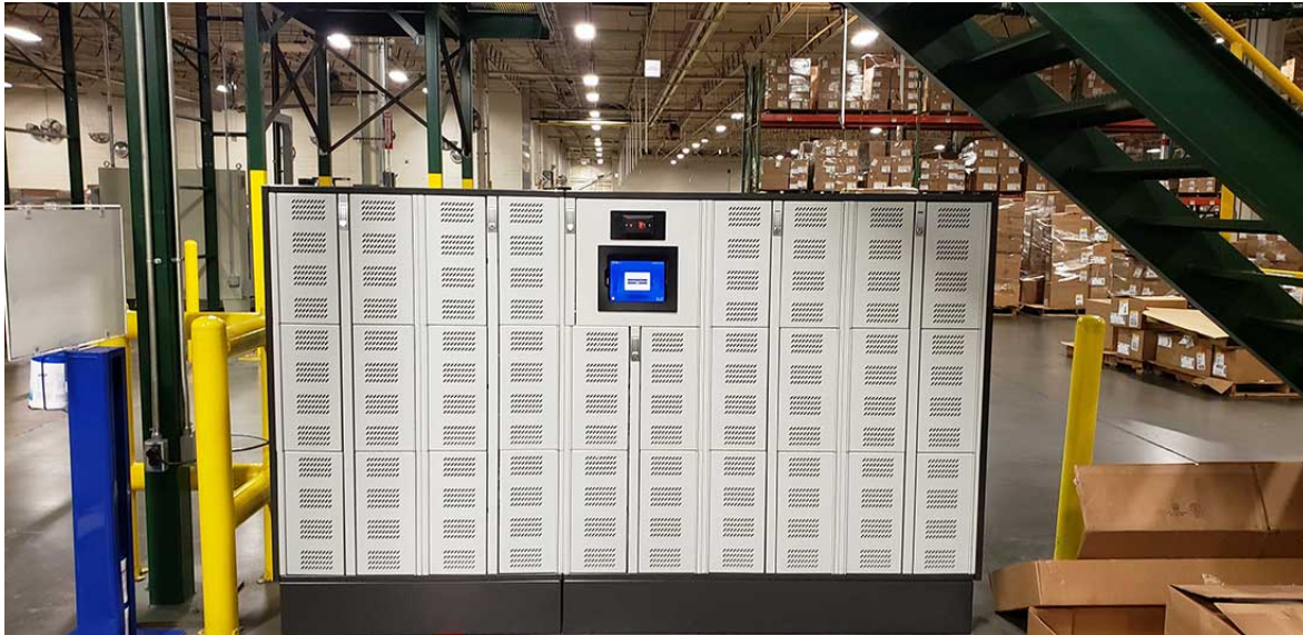
Figure 4.1: RFID-based electronic lockers from Keonn based on the AdvanShelf™ solution [97]
