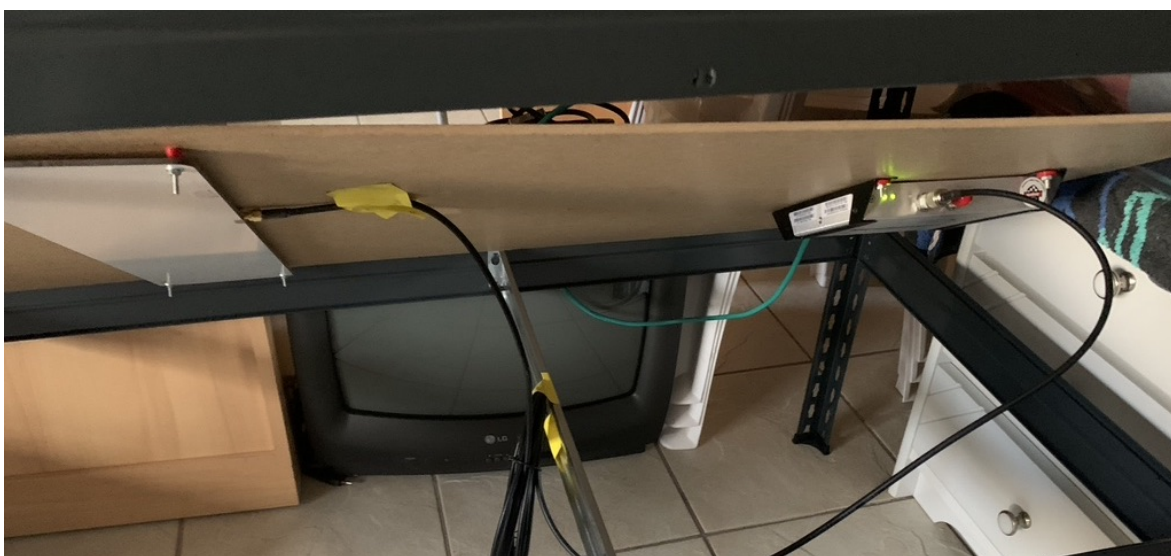
Figure 6.2: Photograph of the Keonn Advantenna-p14 and Impinj Speedway R120 attached behind the bottom shelf
