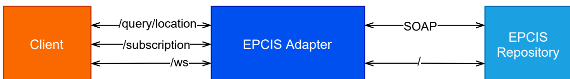
Figure 6.5: Functional block illustration with endpoints of the EPCIS-adapter developed in this dissertation
