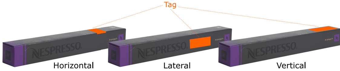
Figure 7.1: Tag orientation tested in this dissertation: horizontal, lateral and vertical, respectively
