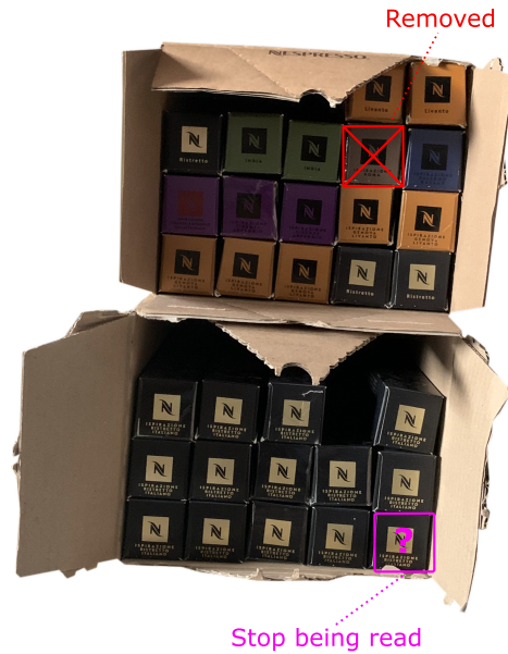
Figure 7.5: Non linear obstruction phenomenon illustrating miss readings caused by the removal of a tagged sleeve
