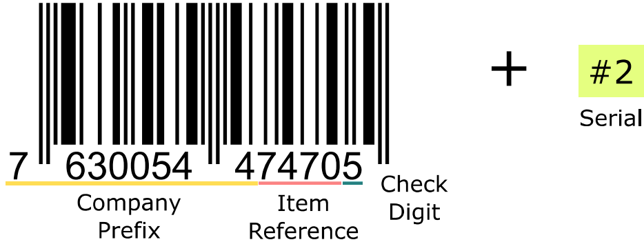
Figure 3.6: Relation and interoperability between SGTIN and barcode's GTIN
