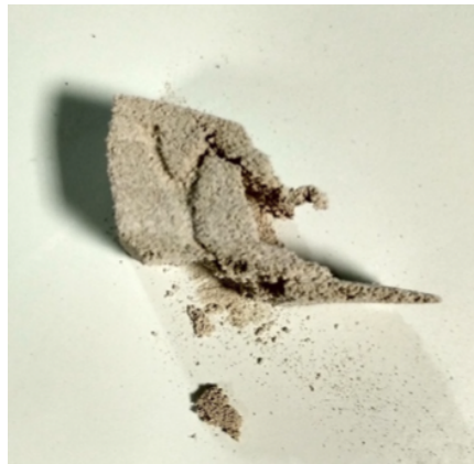
Figure 4.17: Printed part (cube) using T3, T5 and T7 formulations, which have in common the coarse particles of PVA powders.
