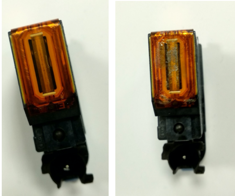
Figure 4.18: Clean (left) and clogged (right) printhead during the binder jet printing of T3, T5 and T7 formulations, which have PVA coarse particles in their composition.
