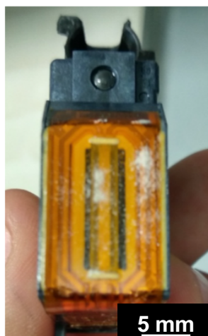
Figure 3.9: Obstructed printhead after binder jet printing of the PP-5CMC feedstock.
