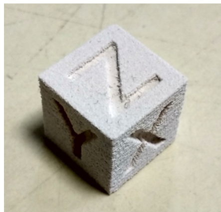
Figure 4.21: Printed part (cube) with the T1 formulation, presenting the highest Hausner Ratio.
