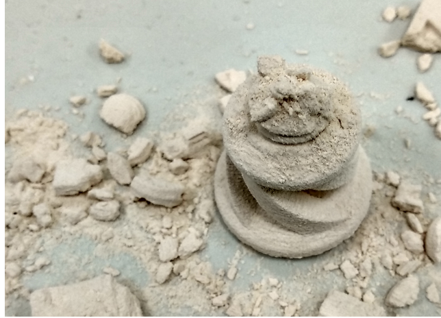
Figure 7.31: Complex part, produced by BJP with 50HT feedstock, after the firing cycle at 980 - 1020 °C for 15 - 18 h.
