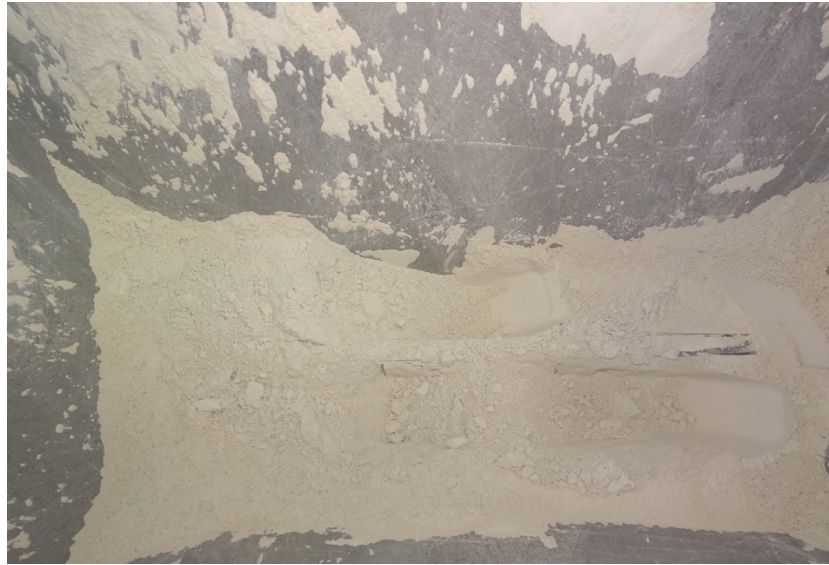
Figure 7.27: Compacted 50HT feedstock powder in the bottom of the feeder, leading to the 60100 error.
