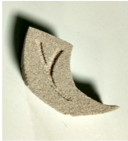
Figure 4.19: Printed part (cube) with T9 formulation, which exhibits the lowest Hausner Ratio and higher flowability.
