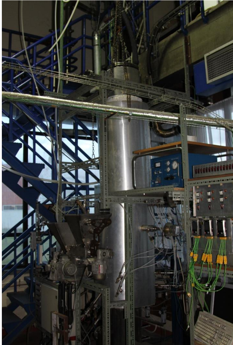
Figure 1.4 – DAO-UA pilot-scale 80kW th BFB reactor.
