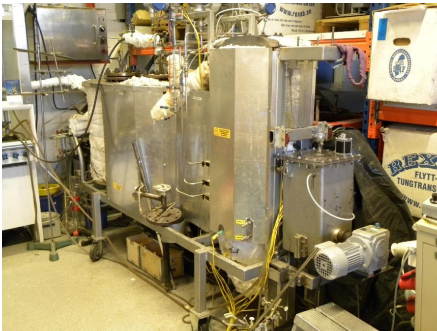
Figure 1.8 – KTH 5 kW th allothermal BFB bench-scale infrastructure.
