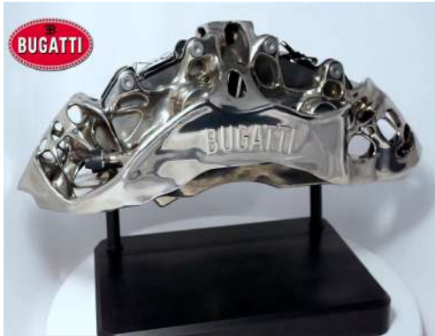
(a) Fabrico do travão do Bugatti Chiron usando Selective Laser Melting (SLM) [4].
