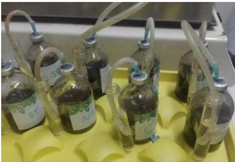
**Figure 9.** Batch experiments setup for short-chain organic acid production.
