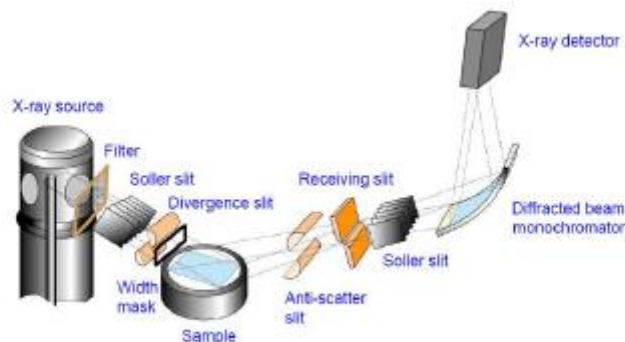
Figure 2.7 – X-Ray operation scheme 70 .
