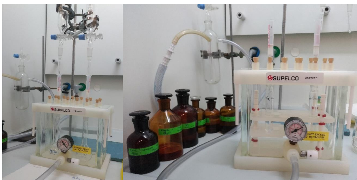
Figure 12 – Solid-phase extraction (SPE) fractionation system consisting of ionic exchange ( \text{NH}_2 ) cartridges adapted to a vacuum manifold, volumetric glass beakers and glass tubes for sample collection.
