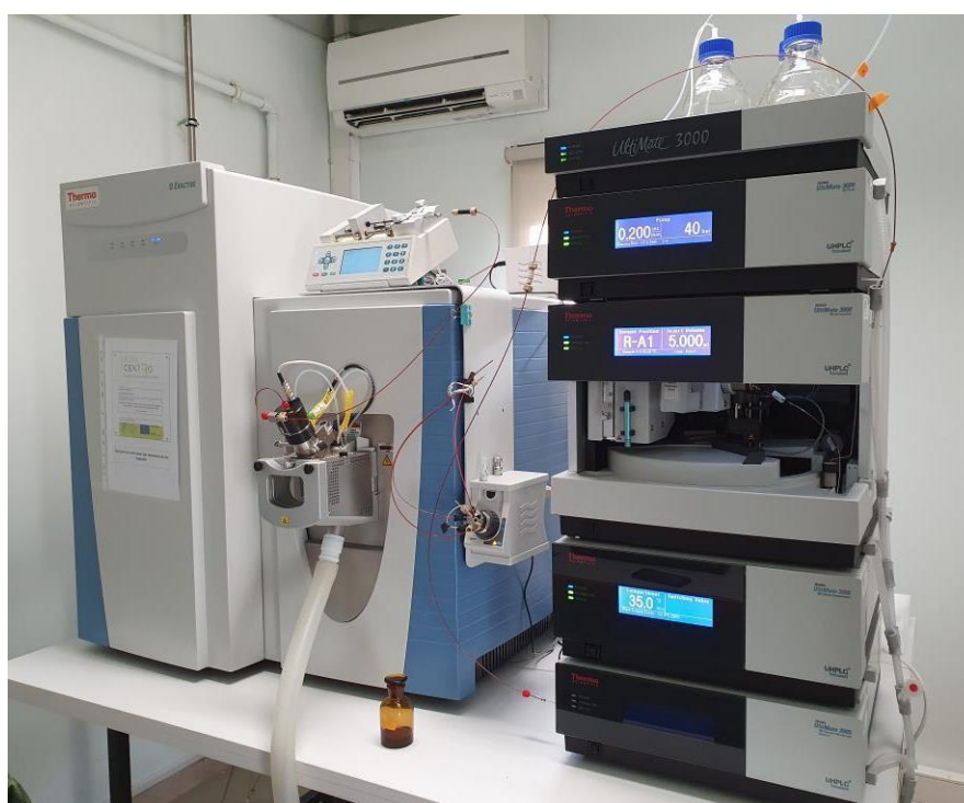
Figure 13 – The High-Performance Liquid Chromatograph (UltiMate 3000™ UHPLC system, Thermo Fisher Scientific, Germering, Germany) (on the right) coupled online to the Q-Exactive Orbitrap mass spectrometer (on the left).
