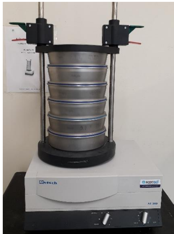
Figura 5. Coluna de peneiros composta por peneiros com as malhas 1000 \mu\text{m} , 500 \mu\text{m} , 212 \mu\text{m} , 125 \mu\text{m} , 63 \mu\text{m} e base.
