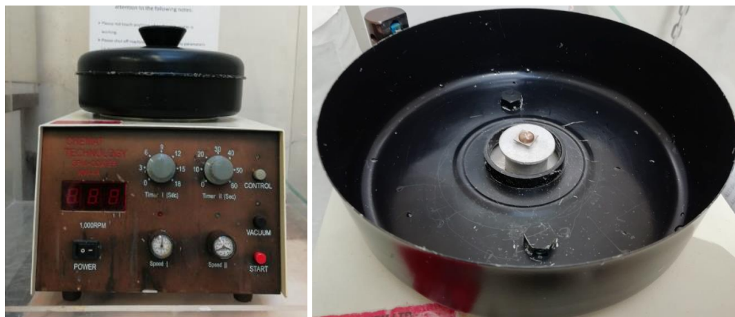
Figure 16. Spin-coater used in the PLLA film deposition.
