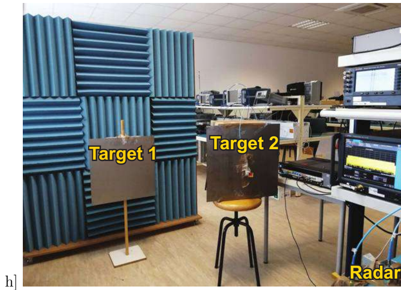
Figure 11.6: Photograph of the scenario with measurement setup and two targets, where the target 2 was equipped with an antenna transmitter.
