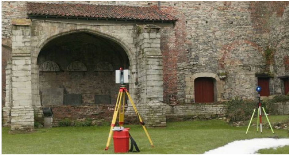
Figure 2.5: TLS system example used for recording the Sint-Baafs Abbey [42]
