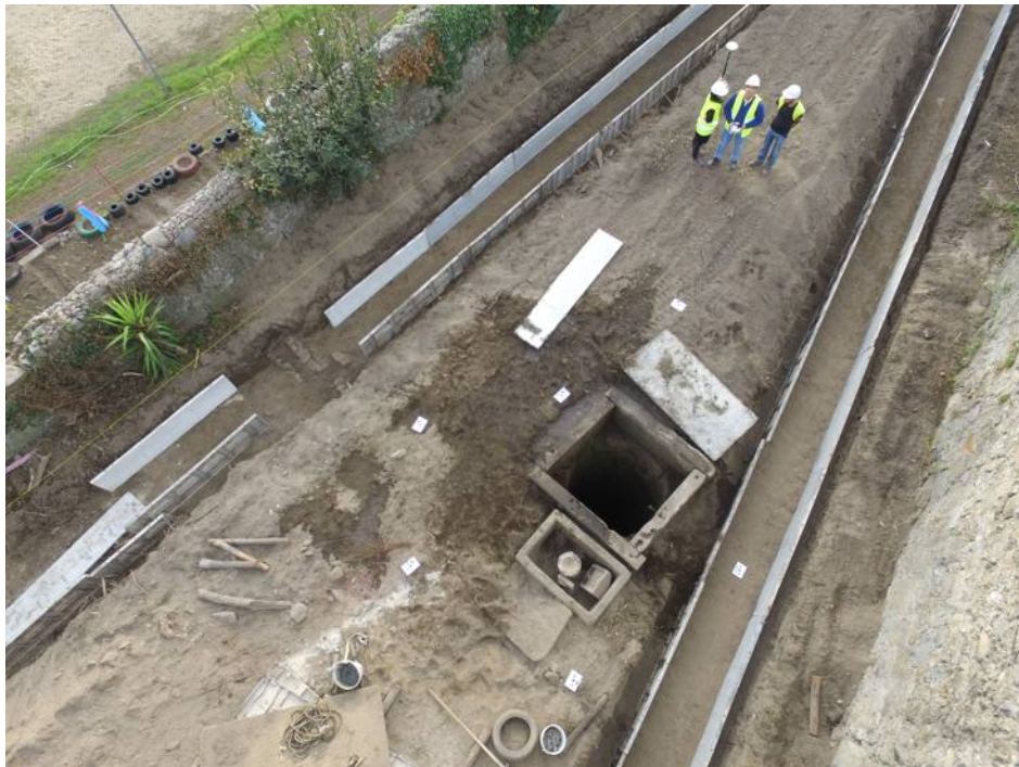
Figure 5.10: Archaeological data acquisition setup using ground control points, UAV and GPS (Courtesy of UAUM)
