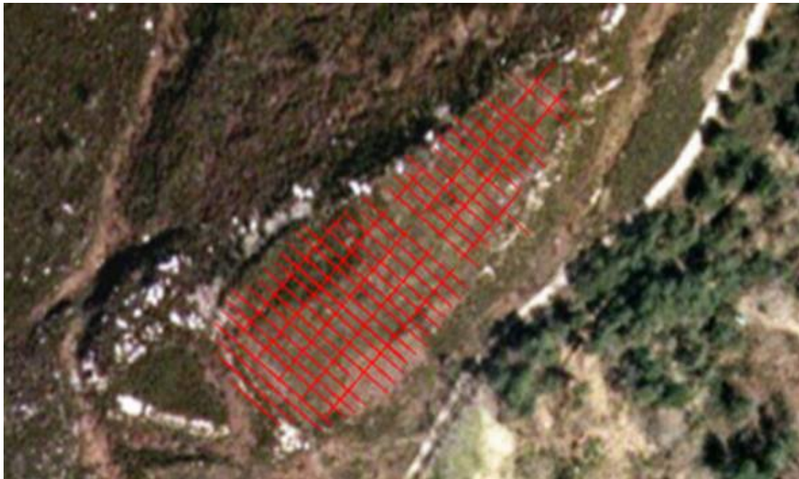
Figure 7.29: Linear grid of the ERT survey
