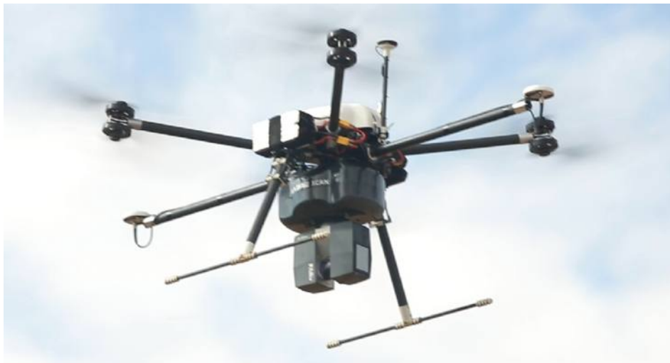
Figure 2.4: ALS system example (LiDAR sensor mounted on an unmanned aerial vehicle )
