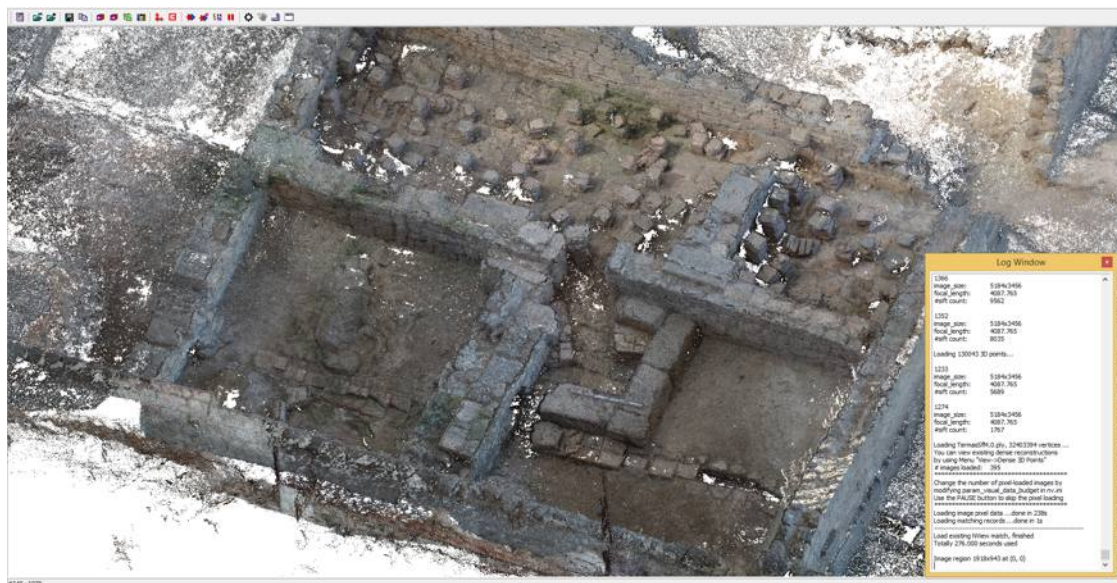
Figure 7.18: Dense 3D point cloud generated with VisualSfM
