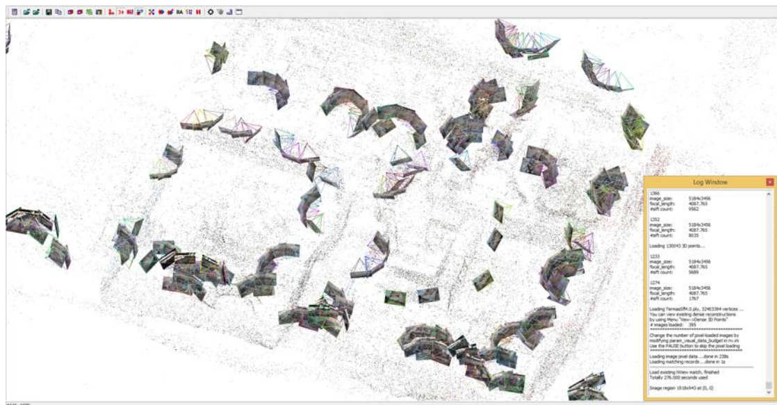
Figure 7.17: Sparse 3D point cloud generated with VisualSfM
