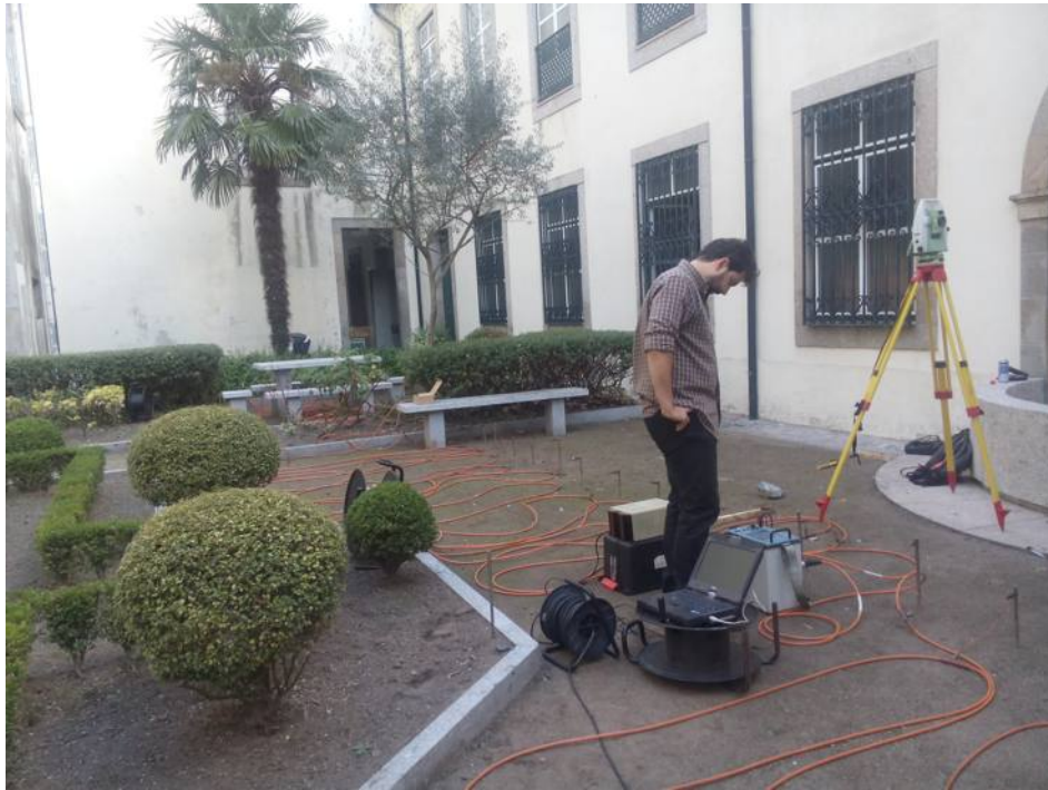
Figure 5.12: ERT data acquisition setup (Courtesy of SINERGEO)
