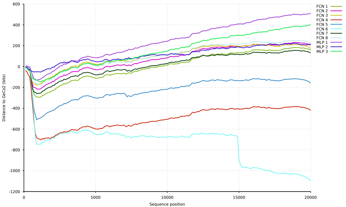
Figure 3.1: Comparison of different neural network architectures. The plot shows the distance to the GeCo2 for the first 20 thousand symbols of the EnIn DNA sequence. Positive distances indicate the network is outputting less bits than GeCo2.
