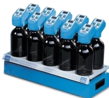
Figure 24| Respirometric BOD system used to determine BOD_5 .
