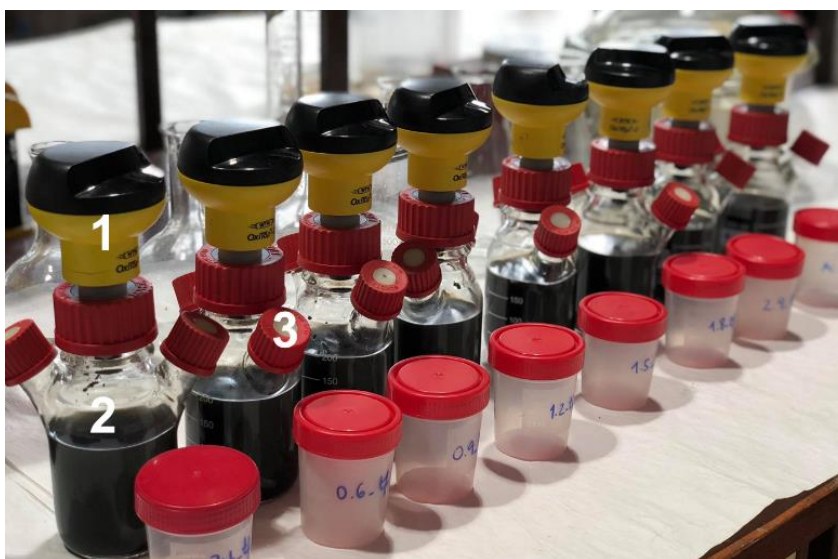
Figure 20| Oxitop system used in batch anaerobic assays and sample flasks. 1) Measuring head; 2) Glass sample vessel; 3) Nozzle and septum seal.
