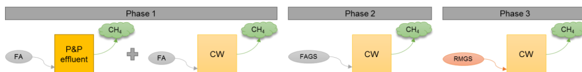
Figure 3| Integration of different types of wastes in waste(water)-to-energy approach, divided into three phases, according to the type of inorganic waste added. In phase 1, the addition of fly ash (FA) powder to the AD of both pulp and paper (P&P) effluent and cheese whey (CW); in phase 2, the addition of fly ash-based GS (FAGS) and in phase 3, the addition of red mud-based GS (RMGS), both to the AD of CW for methane production.
