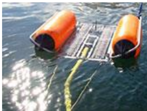
Figure 3.6 – High frequency marine source, Sparker. (from https://www.geomarinesurveysystems.com ).
