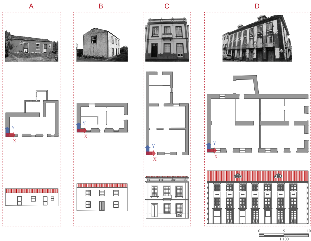
Figure 4.14: Overview of the geometry and building typology of each case study (from A to D): ground floor plans and the respective main façade elevations. Please note that traditional stone masonry elements are coloured in grey, while masonry brick blocks are coloured in light grey. Moreover, the reference axes (X and Y) considered throughout this subsection to each model are identified in the respective ground floor plans.
