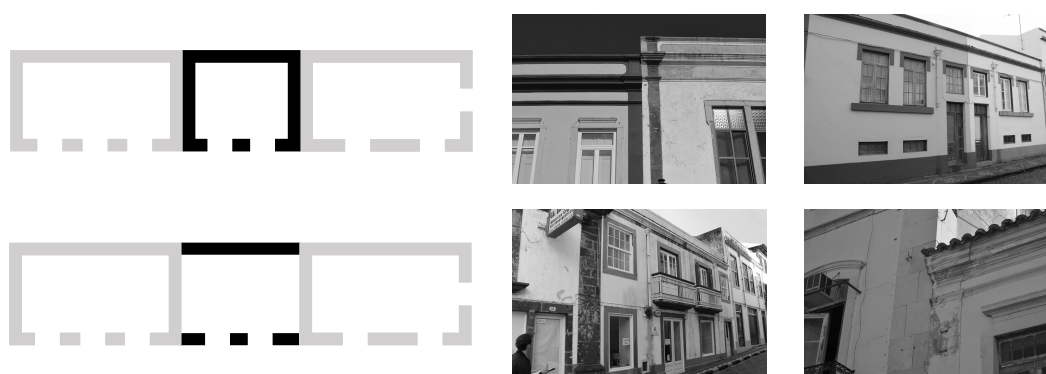
Figure 3.10: Illustration of the two possible configurations of buildings erected in different time periods: pre-existent (in grey) and a new building (in black).
