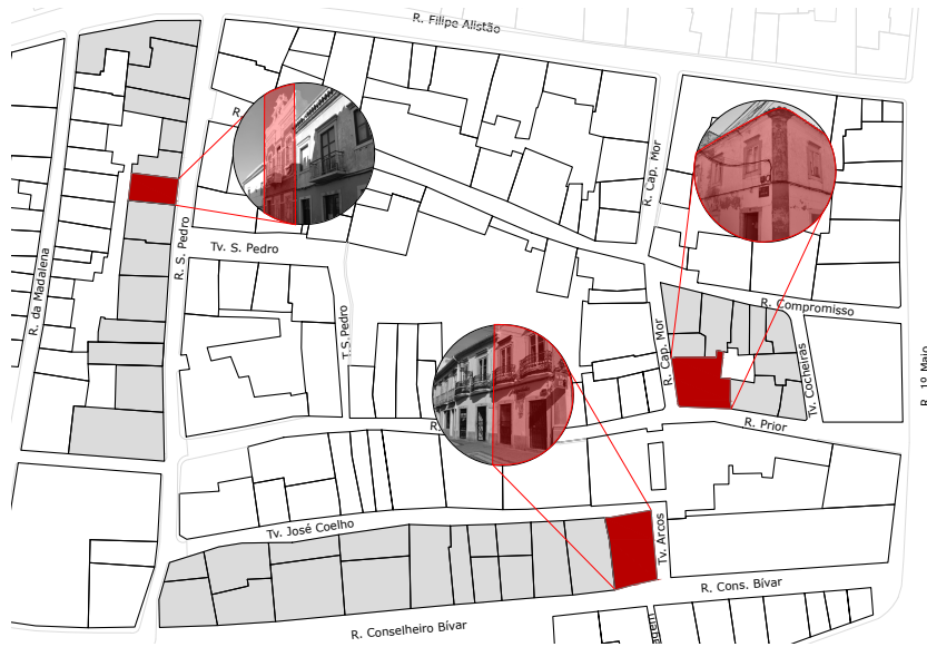
Figure 3.7: Example of the different possible configurations of assets enclosed in aggregate, observed in the historic centre of Faro (in Portugal): mid-row, end-row and corner-end (respectively from left to right).
