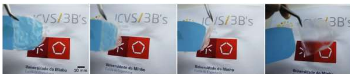
Figure V-2. Detachment of the (CHT/CS) 250 multilayer assembled onto a low surface energy PP substrate: just by pushing through the dry membrane using tweezers, we obtain the freestanding film.
