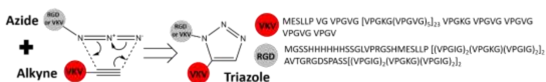
Figure III-1. Chemical scheme representing the click chemistry reaction, that results from the Huisgen 1,3-dipolar cycloaddition of azides and alkynes.
